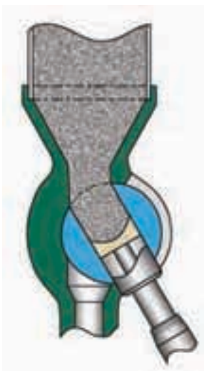
Benchrest proven hemispherical metering chamber cavity.
