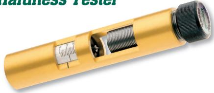
A SAECO Lead Hardness Tester will pay for itself many times over by allowing you to convert inexpensive scrap lead of unknown composition into casting alloy of known and reproduceable hardness. It provides a standard by which you can check the quality of purchased cast bullets. The SAECO Lead Hardness Tester measures alloy hardness by determining the depth of penetration of a hardened steel indenter into a bullet. Relative hardness of the bullet is read off a vernier scale.
